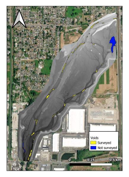
Figure 4. Preliminary DEM for the Countyline project created from the 2022 LiDAR with voids outlined.
