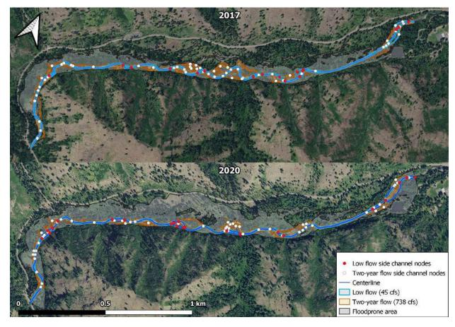
**Figure 28.** Comparison of the water surface extents at low flow, a 2-year flow, and the floodprone area at Tucannon PA-3 in 2017 (pre-project) and 2020 (post-project). Side channel nodes are the junctions between the main channel and each side channel entrance. Base maps are 2017 and 2020 NAIP imagery.
