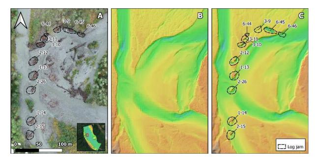
**Figure 6.** Example displaying how constructed log jams (A) were mosaicked with the pre-project LiDAR surface (B) to create an as-built DEM with project design elements included (C).
