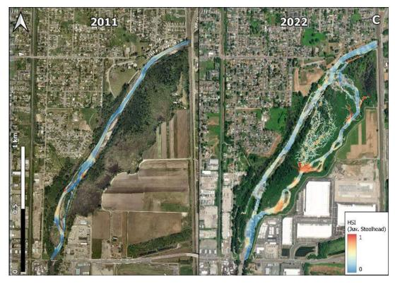
Figure 15. Habitat suitability index results for Countyline at low flow (500 cfs) for juvenile steelhead. Base maps are 2011 (pre-project) and 2021 (post-project) NAIP imagery.
