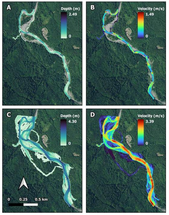
**Figure 20.** Depth and velocity for the Upper/Lower Fobes project site on the South Fork Nooksack River. Panels A and B show the low flow scenario (250 cfs) and panels C and D show the 2-year flow scenario (10,332 cfs).
