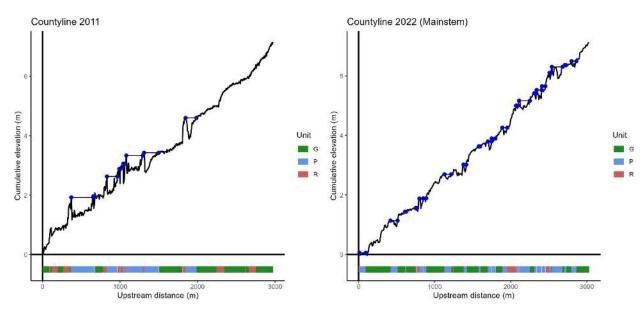
Figure 11. Thalweg long profile and results from habitat classification for Countyline (mainstem only). Habitat unit type definitions are as follows: G = Glide, P = Pool, R = Riffle.
