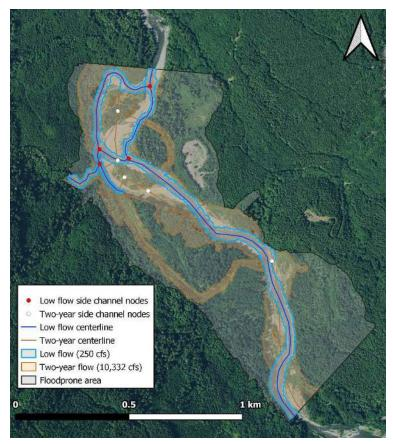
**Figure 19.** Comparison of the water surface extents at low flow, a 2-year flow, and the floodprone area at Upper/Lower Fobes in 2021 (pre-project). Side channel nodes are the junctions between the main channel and each side channel entrance. The base map is 2021 NAIP imagery.
