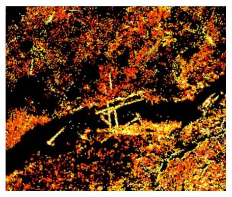
**Figure 2.** Example of a height filtered point cloud ( $0.3 \text{ m} \le Z \le 1 \text{ m}$ ) from Tucannon PA-3 in 2017, colored by intensity. Large wood is identifiable as high intensity (brighter colors) linear segments.
