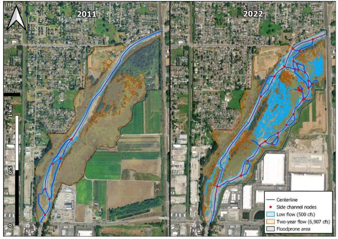
**Figure 9.** Comparison of the water surface extents at low flow and a 2-year flow at Countyline in 2011 and 2022. Side channel nodes are the junctions between the main channel and each side channel entrance. Base maps are 2011 (pre-project) and 2021 (post-project) NAIP imagery.
