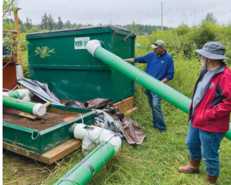
A visitor tours the biofiltration pilot project that may be a valuable tool to fight the threat posed by 6PPD, a chemical found in tires that can be deadly for salmon. Trevor Pyle
